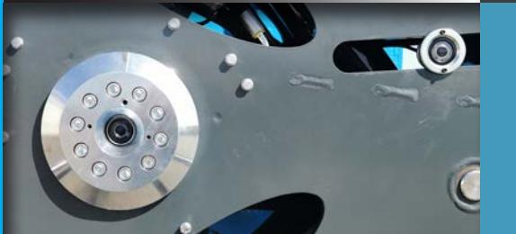
2 Camera System - for hub and bolt alignment
